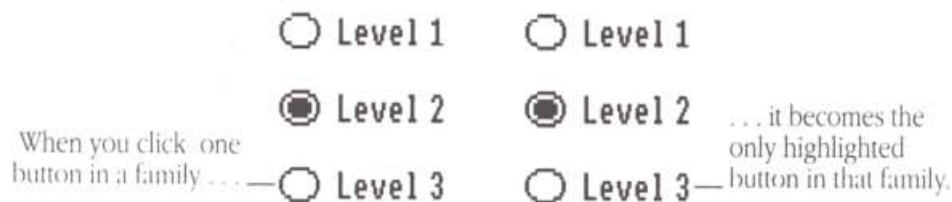
Figure 4-34 The effect of clicking a button that is part of a family
