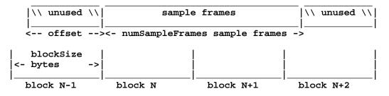
Figure 5-Block-Aligned Sound Data
