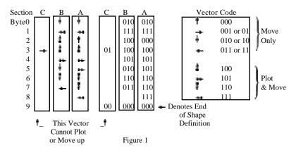
For each vector in the line, determine the bit code and place it in the next available section in the table. If the code will not fit (for example, the vector in section C can't plot a point), or is a 00 (or 000) at the end of a byte, then skip that section and go on to the next. When you have finished coding all your vectors, check your work to make sure it is accurate.
