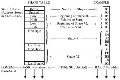
The address of the Shape Table's Start should be stored in locations \$328 and \$329. If the SHLOAD subroutineis used to load the table. start will be set to LOMEM(normally this is at \$0800) and then LOMEM will be moved to one byte after the end of the Shape Table, automatically.
