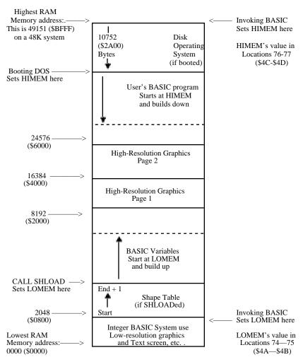
Unfortunately, there is no convention for napping memory. This map shows the highest (largest) address at the top, lowest (smallest) address at the bottom. The naps of Shape Tables that appear on other pages show the Starting address (lowest and smallest) at the top, the Ending address (highest end largest) at the bottom.
