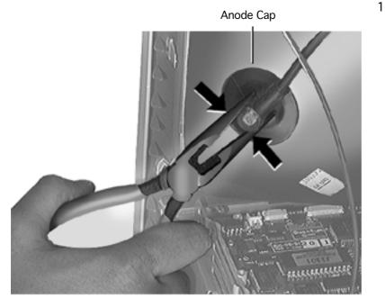
Using needlenose pliers, compress the anode cap to free it from the anode aperture.
