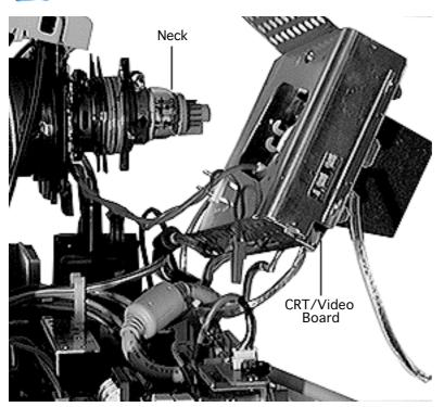
Remove the CRT/video board assembly from the neck of the CRT. Refer to the Take Apart chapter of the monitor or computer manual for steps to remove the CRT/ video board.
