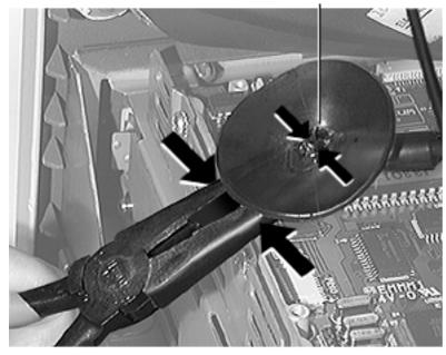
Replacement Note: To replace the anode cap, use needlenose pliers to press together the plastic cup outside of the anode connector so that you can insert it into the anode aperture. After inserting the connector, tug on the high voltage cable to make sure it is firmly seated. Then press down around the edges of the rubber anode cap to ensure a firm seal.
