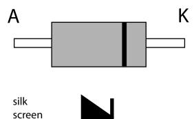
The diode must be oriented correctly. There are two ends, anode and cathode. Be sure that orientation matches the silk screen.
