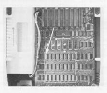
Touch the power-supply cover (the big silver- or gold-colored box along the left side) to discharge any static charge you may be carrying. You need not worry about getting a shock if your Apple is properly grounded, as all high voltages are well insulated inside the grounded power-supply case. (Besides, you have already turned the Apple off, haven't you?)
