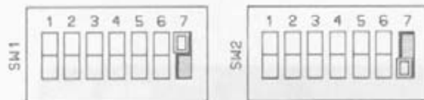
Figure 2-17. RS232C Switch Settings
