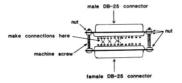
Earlier versions of the 7710 manual were missing two of the the necessary connections: the 4 to 5 and the 20 to 6 connection.
