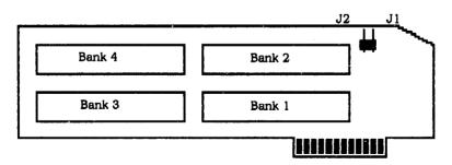
When you add expansion memory, make sure you add memory only in sets of 8 chips starting with bank 1, then bank 2, and so on. Run the memory test program again any time you expand the memory of your Juice Plus board.
