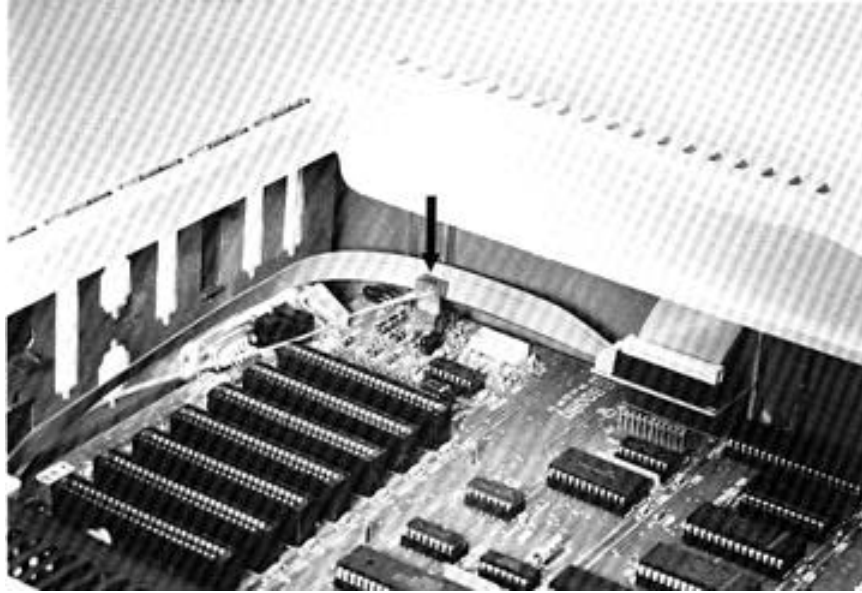
Composite Video Cable connected
