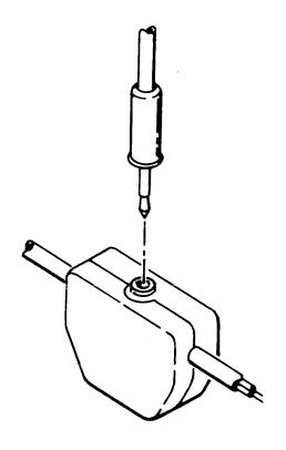
OCS II: Plug the free end of the drop cable into a trunk adapter.
