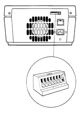
Use a ballpoint pen to set the switches for one of the addresses listed in the table *Network Device Addresses* below. Set them for address 0 if this is the first or only Omnidrive on your network. One Omnidrive should always be set to address 0.
