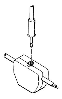
OCS II: Plug the other end of the drop cable into a trunk adapter.
