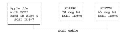
Note that the SCSI card itself has a SCSI ID number of 7. The ST277N, of the two drives, has the higher SCSI ID number. Because of this, if I have 1 partition on this drive, it appears as slot 5, drive 1 and any partitions on the other drive appear as slot 5, drive 2, then the next (if there is another) would be slot 2, drive 1, then the next partition (again, if one exists) on the ST225N would be slot 2, drive 2.
