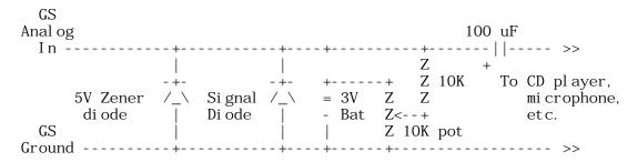
The Ensoniq is designed to handle 0 to 2.5V input, but audio sources usually swing more or less equally +/- about zero. Therefore we need a level shifter, to put the appropriate DC bias onto the input. The 3V battery and the 10K pot are for this. To stop the low internal impedence of the battery effectively shorting the sound source (which happens with the first circuit), I've included another 10K resistor.
