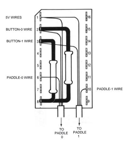
Figure 7.11 Wiring a paddle set plug
