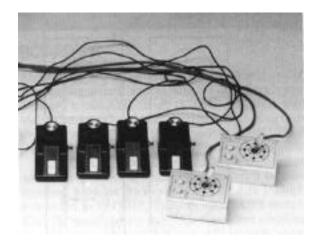
Figure 7.12 This Game I/O Extender can Support Two Sets of Paddlea and Two Joysticks Simultaniously
