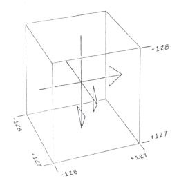
The above diagram shows the limits for each of the three coordinates. Note that these limits define a "cube of space", 256 units along each side. All 3-D objects reside in this space. When more than one object is being displayed, each object has its own 3-D space, though these spaces may overlap or even coincide on the screen.
